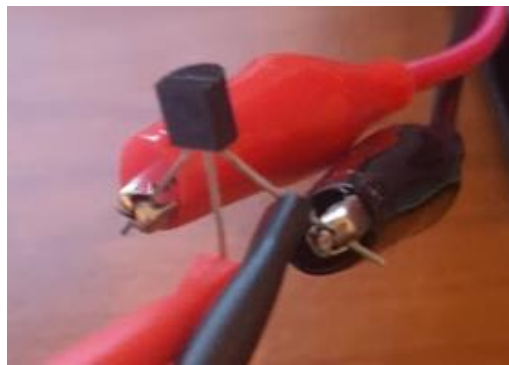
Figure 50: Testing temperature sensor
